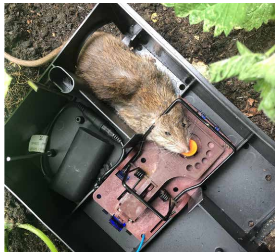
Example of capture of grown rat in break-back trap with waterproof digital 24/7 sensor for outdoor
